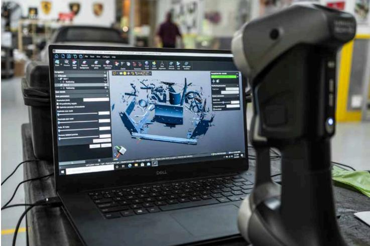
The car is scanned to obtain a digital mesh of the complete exhaust envelope. Attention must be paid specifically to the original mounting points, areas of tight clearances and factory inlets and outlets to ensure that the exhaust system will effortlessly fit up to any factory exhaust components up stream and mount using factory hangers and heat shields.
