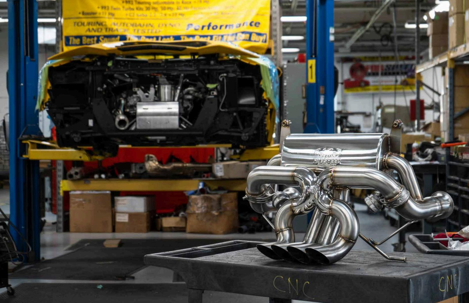
The completed exhaust is installed and tested. Just like when the car originally came into the shop 10 days prior, the car is again dyno tested as well as road tested for any unexpected negative attributes in performance or sound. This testing is down in low and high load scenarios to insure a thorough investigation of driving scenarios.
